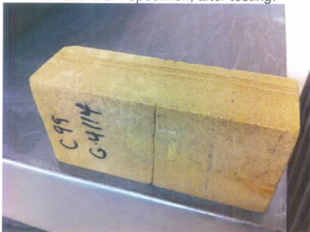
Photo of C99 MOR Specimen, after testing:
