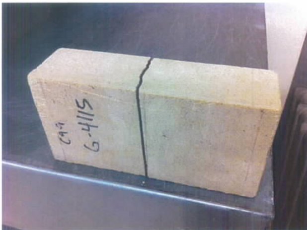
Photo of C99 MOR Specimen, after testing:
