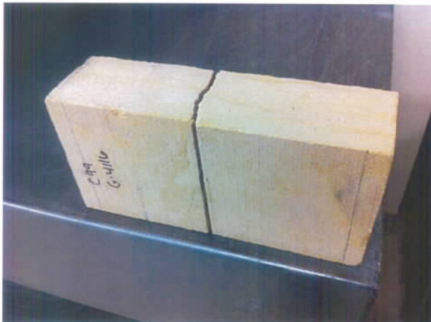
Photo of C99 MOR Specimen, after testing:
